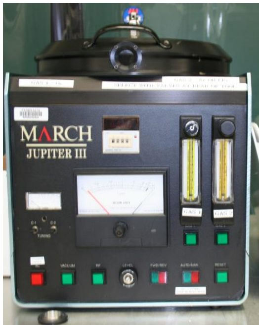
Figure 1: Image of the March Jupiter III RIE system
